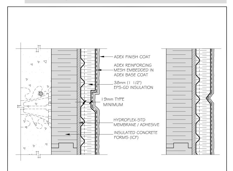
NOTE: AESTHETIC JOINTS SHALL NOT BE LOCATED AT THE CORNERS OF OPENINGS OR AT INSULATION PANEL JOINTS AND SHOULD ALWAYS ALLOW FOR WATER EVACUATION.
